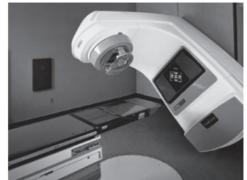
Figure 1: Varian Clinac 2100C. The gantry of the Varian Clinac 2100C linear accelerator can be rotated 360 degrees to deliver radiation from any angle.
